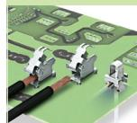
This low-cost, single-pole, metal body uses spring-wire termination as a more secure alternative to wire-to-board soldering. 50-percent lower height offers unrestricted voltage rating at currents up to 30 A.
