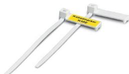
Cable marker carrier, white, unlabeled, mounting type: Assembly with cable ties, cable diameter: > 5 mm, lettering field size: 20 x 8 mm
