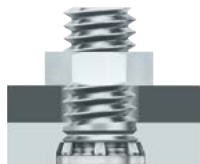
Flush, low-displacement head studs Types FHL/FHLS
