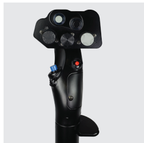
G2: Helicopter Flight Control Grip
