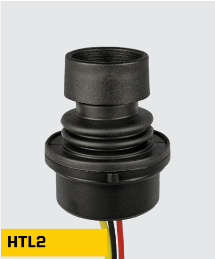
HTL2: Single axis, linear Hall effect, tall concave stadium button
