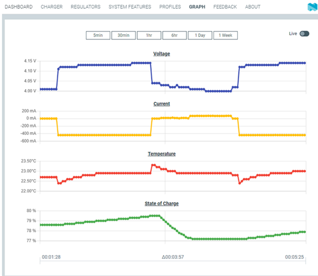
Figure 2: Evaluating the battery model in nPM PowerUP
