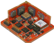
MTi-G-710 OEM: 37x33x12 mm, 11g, 16-pins header
