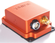
MTi-G-710 encased: 57x42x23.5 mm, 55g, 9-pins push-pull connector
