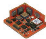
MTi OEM: 37x33x12 mm, 11g, 16-pins header
