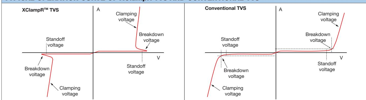
XClampR TVS is a snapback type TVS with an extremely low clamping voltage ratio for suppressing transient voltage to a lower clamping voltage, compared to conventional TVS.
