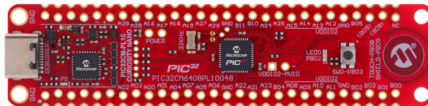
Figure 2-1. Overview of the PIC32CM Curiosity Nano Evaluation Kit
