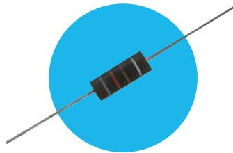
TT Electronics can advise on the exact energy rating required, but 25J at 1K falling to 2.5J at 10K are typical values for leadset protection, and this calls for a composition technology product such as CC series. For PCB mounted resistors offering secondary protection, pulse withstanding thick-film products such as PWC and DSC series are used.
