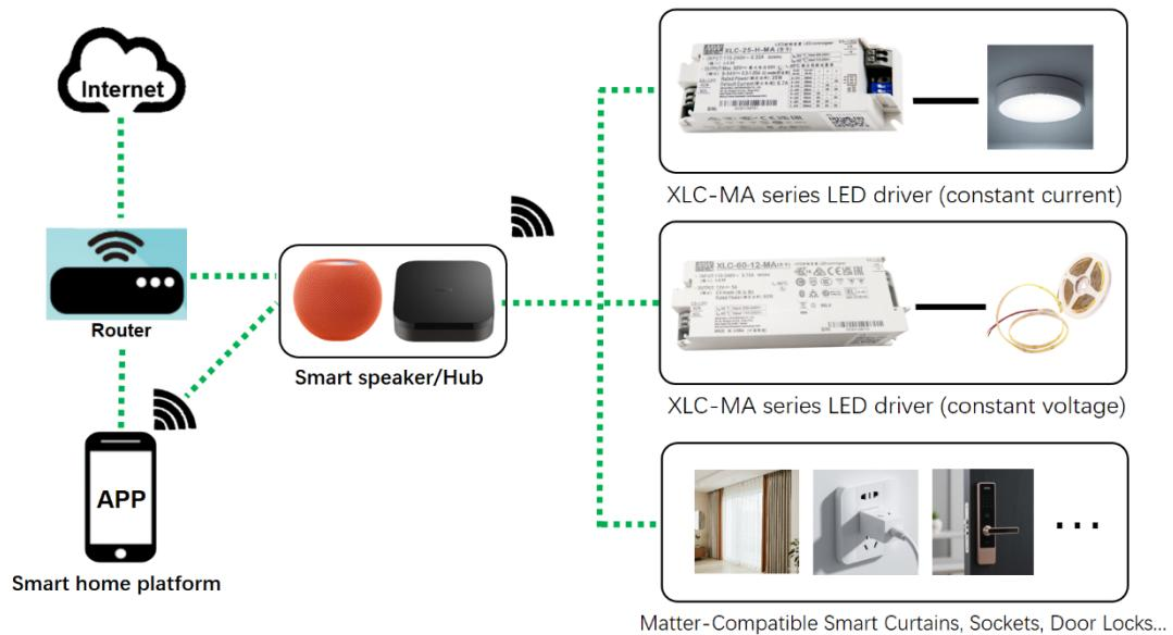
Figure 1: Matter Smart Home Application Diagram
