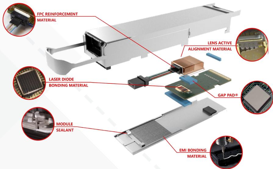
The effective use of advanced materials in an optical transceiver is shown in the diagram above.
