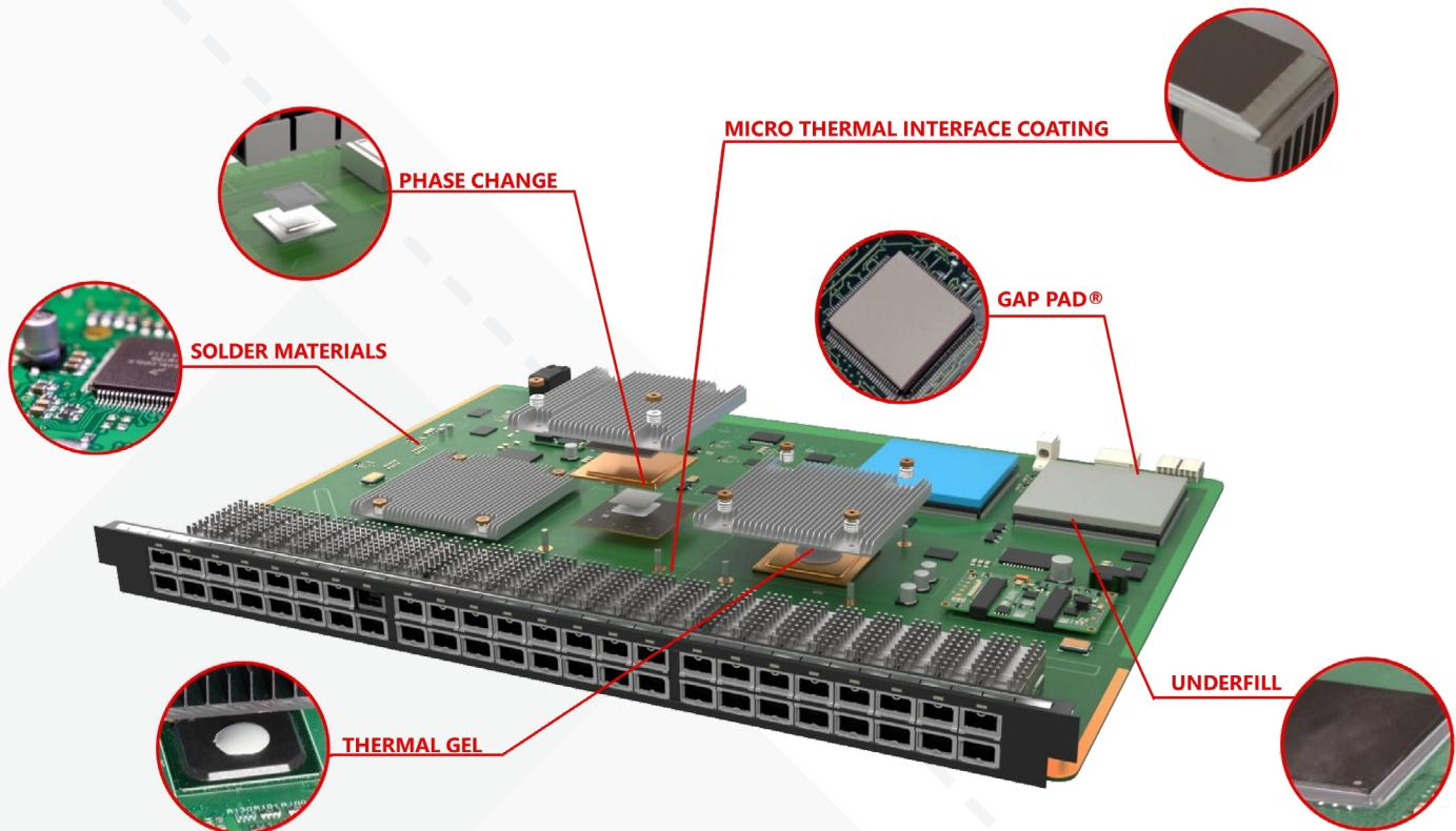
Above is a diagram example of how advanced materials can be used in a circuit board configuration to keep it at maximum operating capacity and performance.
