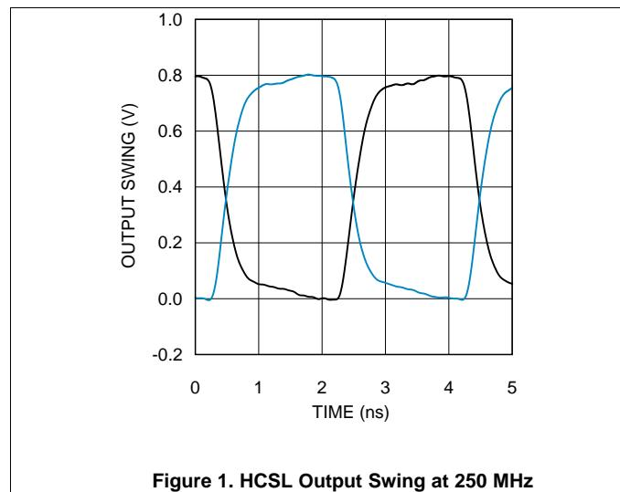
Figure 1. HCSL Output Swing at 250 MHz
