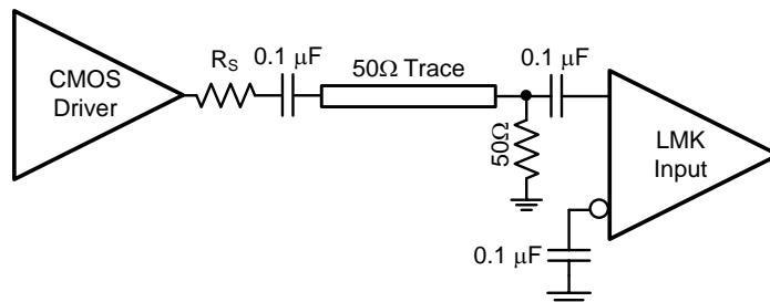
Figure 15. Single-Ended LVCMS Input, AC Coupling
