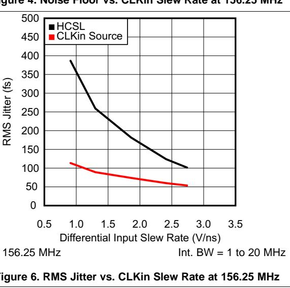
Figure 6. RMS Jitter vs. CLKin Slew Rate at 156.25 MHz
