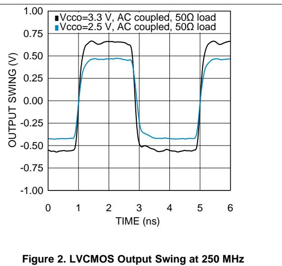
Figure 2. LVCMS Output Swing at 250 MHz
