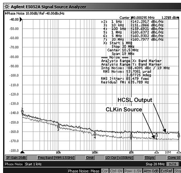
Figure 20. HCSL Phase Noise at 100 MHz
