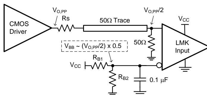
Figure 16. Single-Ended LVCMS Input, DC Coupling With Common-Mode Biasing
