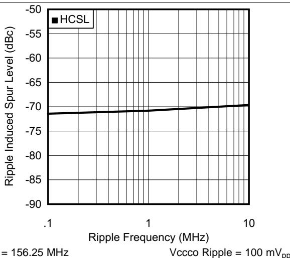
Figure 7. PSRR vs. Ripple Frequency at 156.25 MHz
