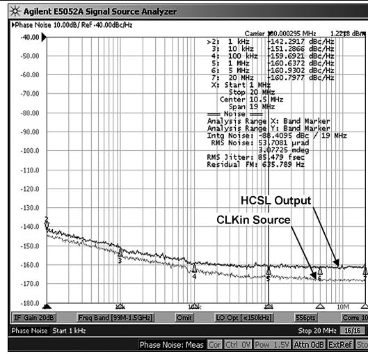
Figure 11. HCSL Phase Noise at 100 MHz
