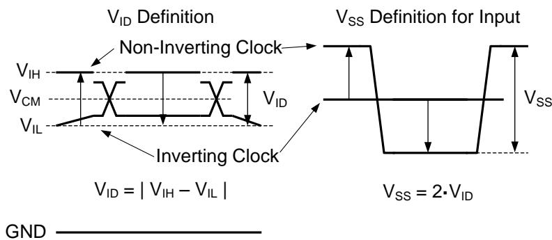
**Figure 12. Two Different Definitions for Differential Input Signals**
