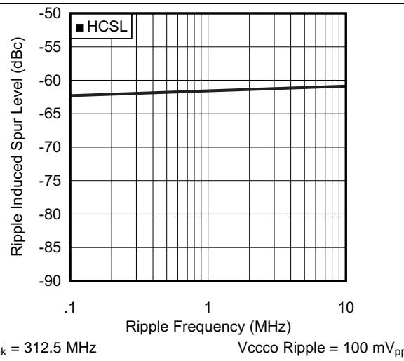
Figure 8. PSRR vs. Ripple Frequency at 312.5 MHz
