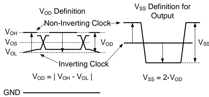
**Figure 13. Two Different Definitions for Differential Output Signals**
