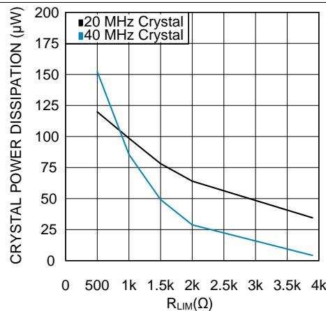
Figure 10. Crystal Power Dissipation vs.  $R_{\text{LIM}}$
