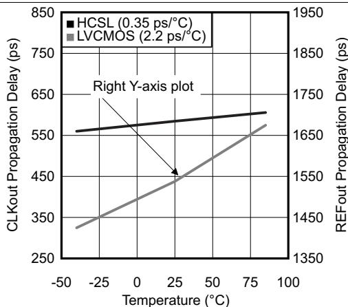
Figure 9. Propagation Delay vs. Temperature
