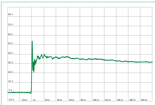
ISO10605 Contact Discharge Plot at +8 kV
