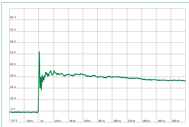
ISO10605 Contact Discharge Plot at +8 kV
