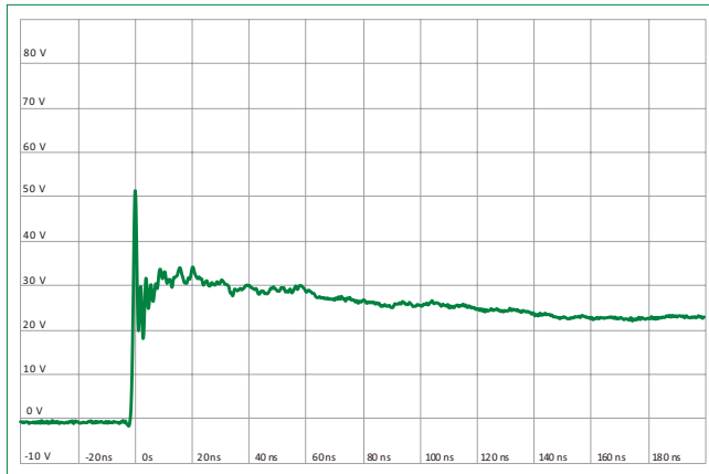
IEC 61000-4-2 +8 kV Contact ESD Clamping Voltage
