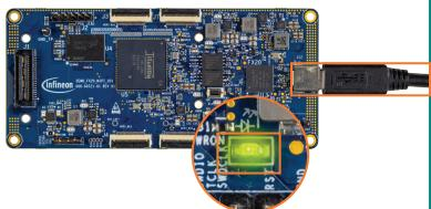
1 Kit connected to PC via USB-C cable and power ON LED glows green
