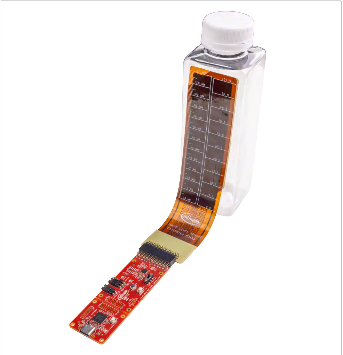
Figure 55 Liquid level sensing setup with container
