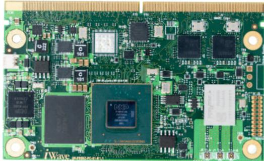
The i.MX 95 SoC based SMARC System On Module is designed as per SMARC specification v2.1.1. It integrates NXP's i.MX 95 offerings, 6x Arm Cortex A55 @ 1.8GHz, 1x Arm Cortex-M33, 1x Arm Cortex-M7, NPU with up to 2.0 TOP/s and IEEE 802.11 a/b/g/n/ac/ax Wi Fi + Bluetooth 5.3 module.
