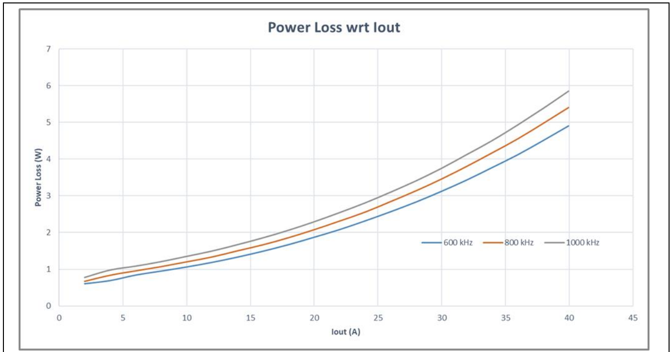
Figure 21 Power loss versus load current without airflow in FCCM with external V CC (12 V in , 1.2 V out , no air flow, 150nH, 600 kHz/800 kHz/1000 kHz, T a = 25 °C)
