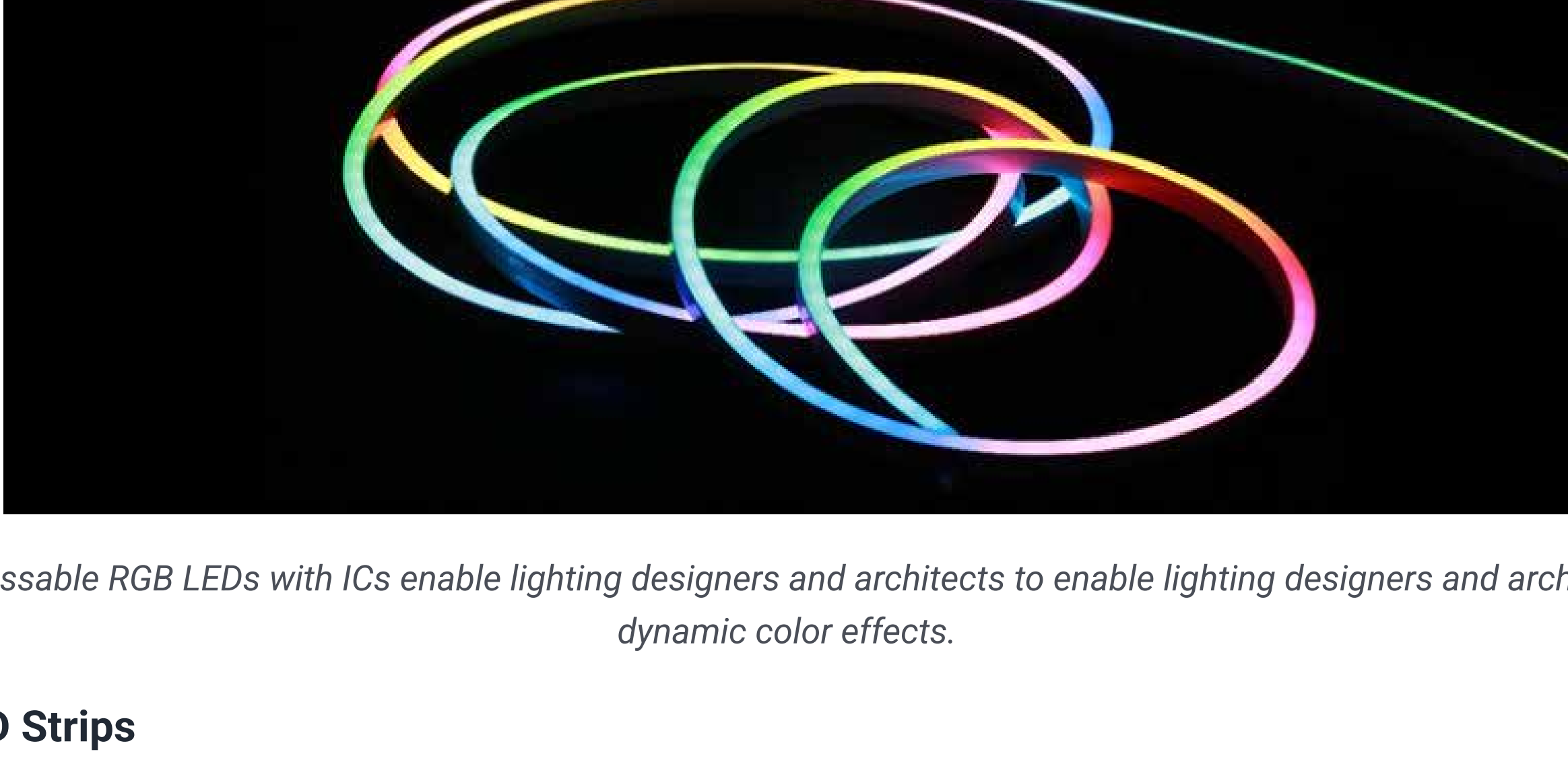
Figure 3: Independently addressable RGB LEDs with ICs enable lighting designers and architects to enable lighting designers and architects to create sophisticated, dynamic color effects.
