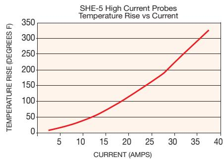
1. For SH-5 Series only 2. Smiths Interconnect's current ratings are defined as the maximum current at which the temperature rise of the probe does not exceed 144°F (80°C) for a single probe in free air at ambient temperature for one hour. Dimensions are in inches (mm) | All specifications are subject to change
