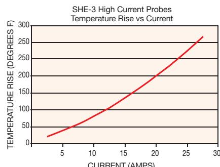
1. For SH-3 Series only 2. Smiths Interconnect's current ratings are defined as the maximum current at which the temperature rise of the probe does not exceed 144°F (80°C) for a single probe in free air at ambient temperature for one hour. Dimensions are in inches (mm) | All specifications are subject to change
