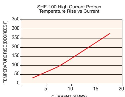
1. For SH-100 Series only   2. Smiths Interconnect's current ratings are defined as the maximum current at which the temperature rise of the probe does not exceed 144°F (80°C) for a single probe in free air at ambient temperature for one hour. Dimensions are in inches (mm) | All specifications are subject to change
