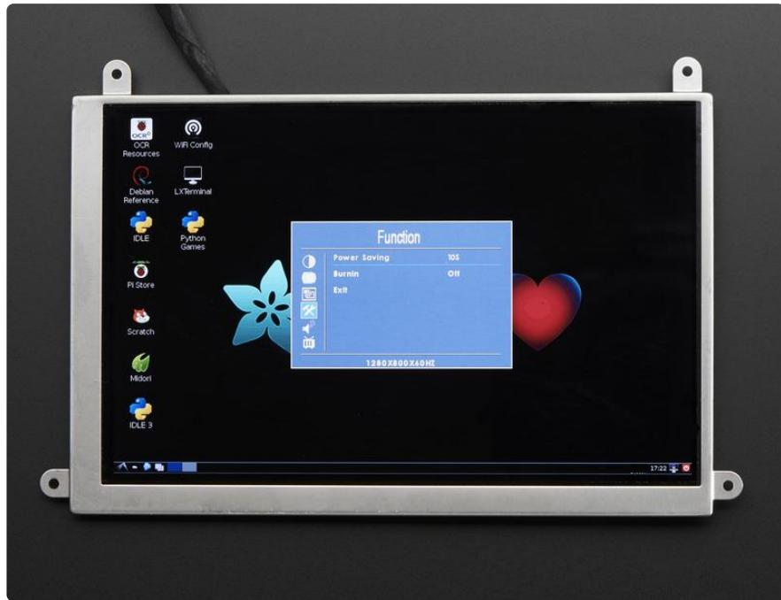
Power Saving - 10s to 60s - how long it takes for the screen to shut off
