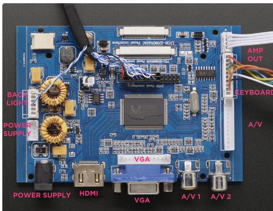
The Power, VGA and A/V JST ports are good alternatives to the main inputs if you don't want bulky cables coming out the sides of your driver board.
