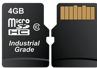
RMPET, a 4D Systems Tool found in the Workshop5 IDE, is capable of repartitioning and formatting microSD cards for FAT16, to be the appropriate type and format. This tool should be used for all cards as it also employs an offset which is critical when using Industrial microSD cards which feature Read Disturb Prevention firmware, which is a special firmware inside the microSD card designed to prevent Read Disturb occurring on NAND based Flash media. Further, discussed in the note.
