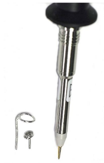
Figure 10. Created simplified probe tip adapter
