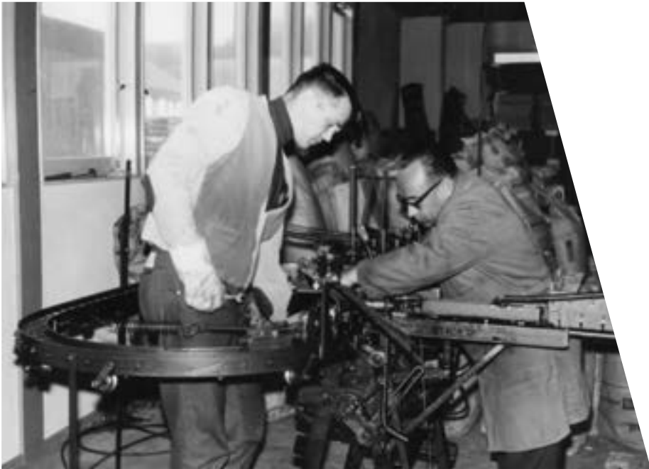
World's first machine for the production of double offset springs
