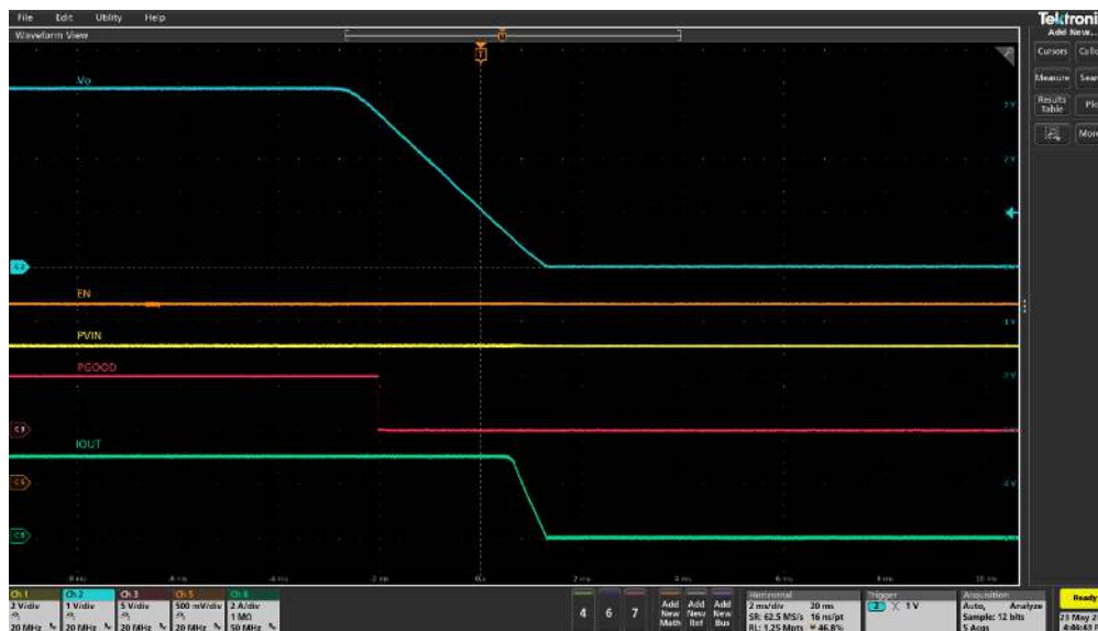
Figure 16 Soft turn off at 3A load (Ch1: PV_{IN} , Ch2: V_{OUT} , Ch3: PG, Ch5: Enable, Ch8: I_{OUT} )
