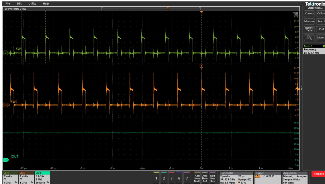
Figure 22 Switch node waveforms at 25A
