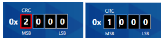
Figure 4. HEX text field, Left: Wrong CRC; Right: Correct CRC
