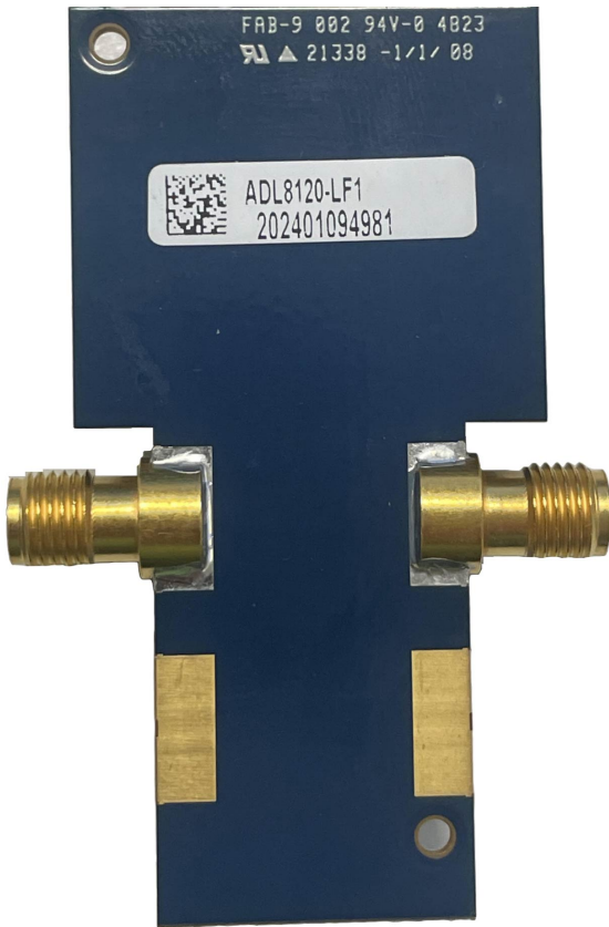
Figure 4. ADL8120-EVAL1Z Bottom Side (30 kHz to 20 GHz Evaluation Board)
