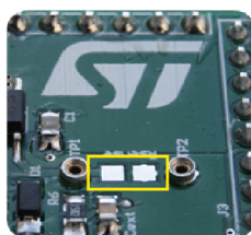
Figure 5. Pads for soldering SMD resistor
