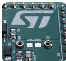
Figure 4. Mounting through-hole sense resistor
