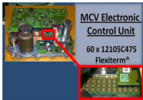
Figure 7: Example MLCC Application in Automotive ECU
