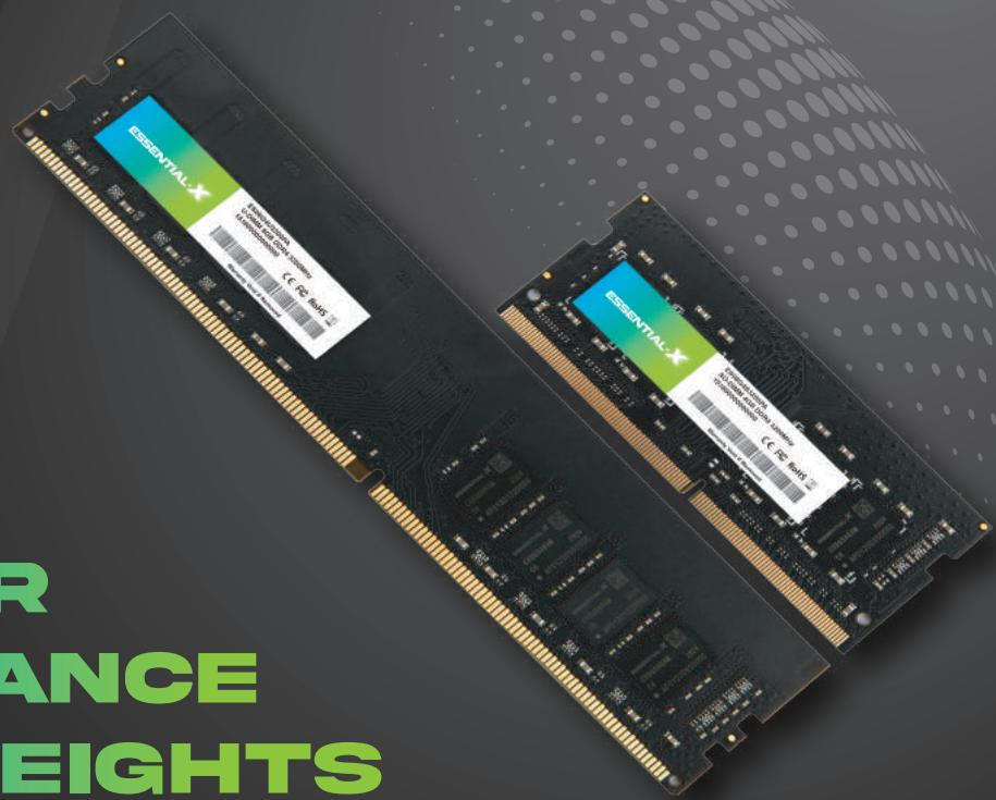
The Essential-X DDR4 3200/2666 RAM modules offer blazing-fast speed and unwavering reliability – making them the ultimate choice for taking your PC's performance to the next level. Available in both the standard and small-outline DIMM form factors, these top-performers will breathe new life into your desktop and laptop computers.
