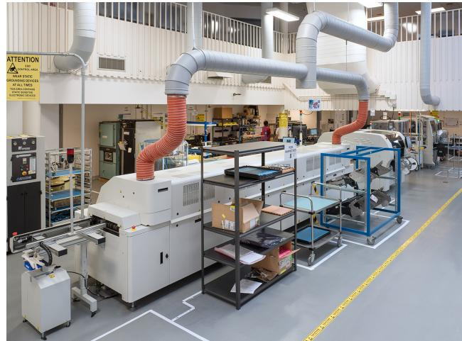
PC board and sub rack assembly. Automation typically translates to high quality assemblies, particularly for connectors designed for rugged or demanding applications. Being able to process special board materials, board thicknesses and board sizes are also a big benefit especially for backplane applications.
