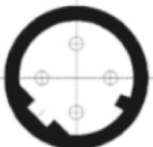
D - Polarization (4 Pin for Industrial Ethernet, Fast Ethernet 100 Mbit/s)
