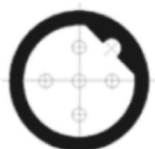
B - Polarization (fieldbus applications like Profibus, Interbus)
