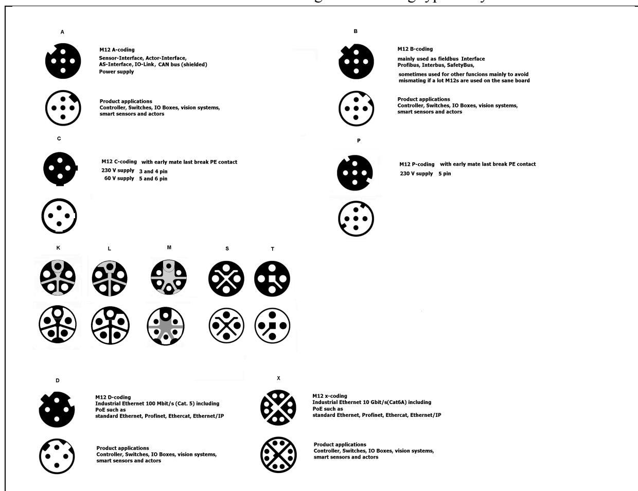
**Polarizations according to IEC 61076-2-101 for M12 male connectors**
