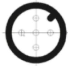
A - Polarization (sensor/actuator applications, DeviceNet CANopen)
