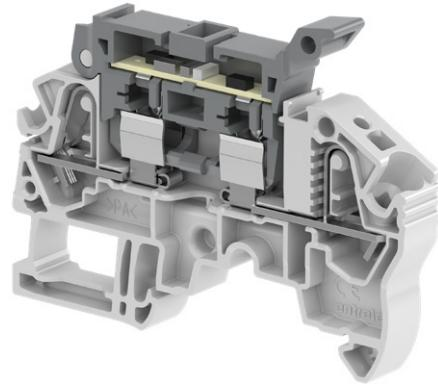
Snk fuse-holder connections terminal blocks are offering world-class certifications with patented pi-spring connection (push-in and spring mode) that helps fast wiring, and faster accessories mounting for 5x20 and 5x25 mm fuses pi-spring (push-in & spring) technology with 4 mm<sup>2</sup> cable size.
