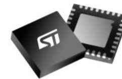
VFQFPN32 5x5x1mm (exposed pad down)
