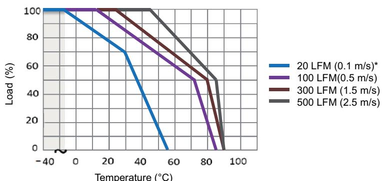
The derating curve was measured at 12 V input and 5 V output.
