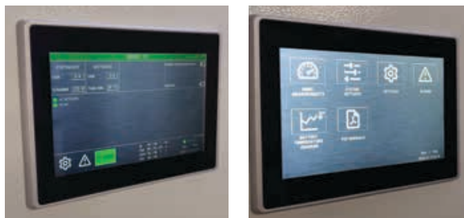
The XV300 HMI PLC offers advanced graphics and allows operations to be loaded very quickly, even when the pages are highly detailed.
