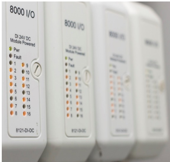
Figure 1. 24V Programmable Logic Controller Input/Output Module
