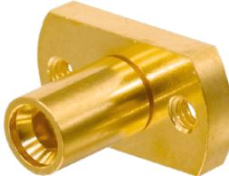
Maximum VSWR of 1.50 out to 65 GHz; Insertion loss of  $0.12\sqrt{F}$  dB Max (F in GHz).
