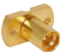
SMA maximum VSWR of 1.20 out to 26.5 GHz; Insertion loss of  $0.12\sqrt{F}$  dB Max (F in GHz)
