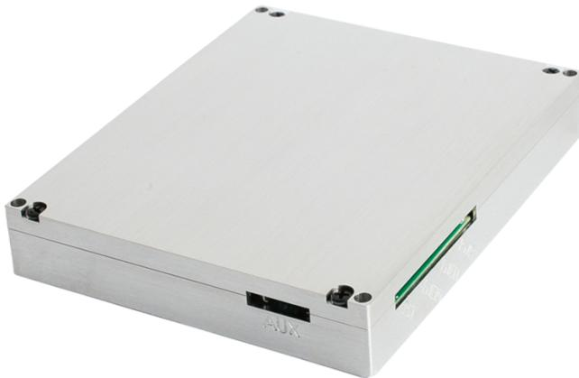
The Smart Radio is an advanced 2x2 MIMO mesh router designed for Industrial IoT applications.
