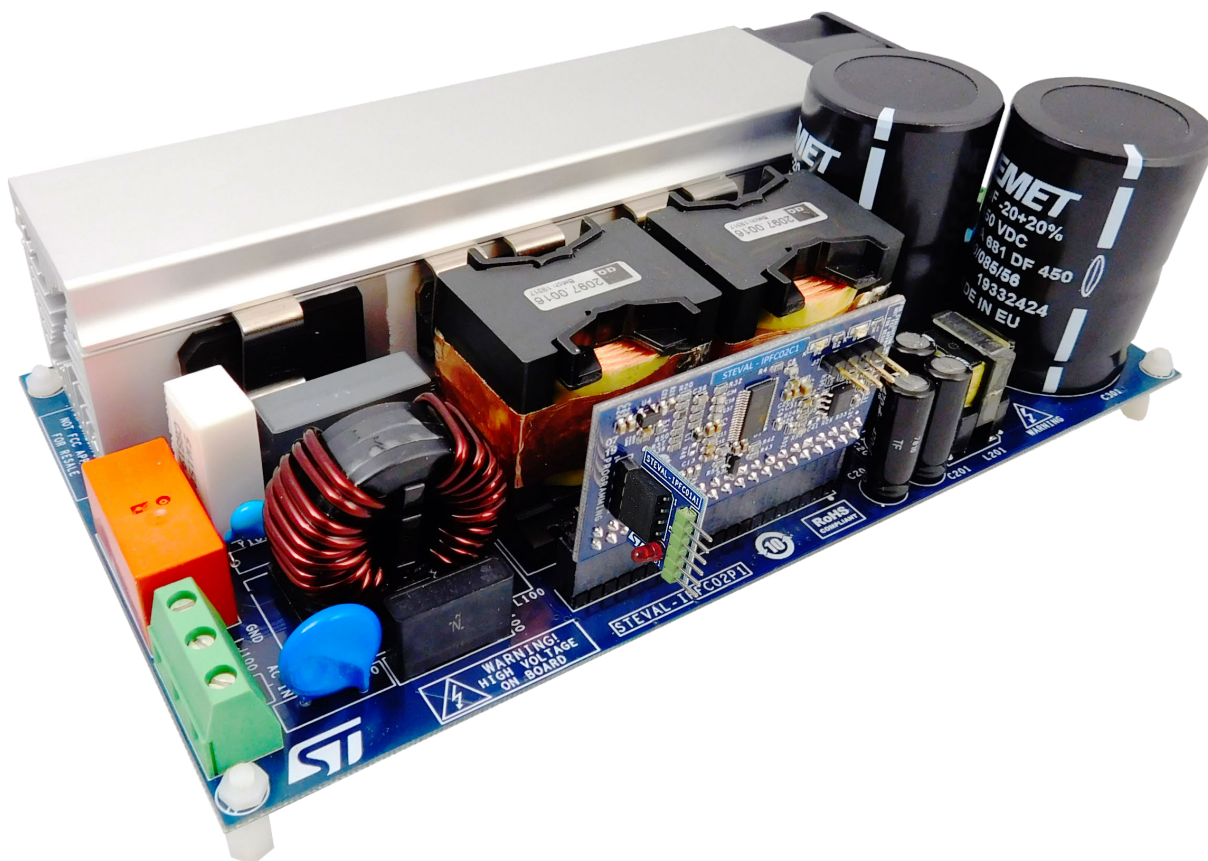
Figure 1. STEVAL-IPFC02V1 evaluation kit with power, control and adapter boards
