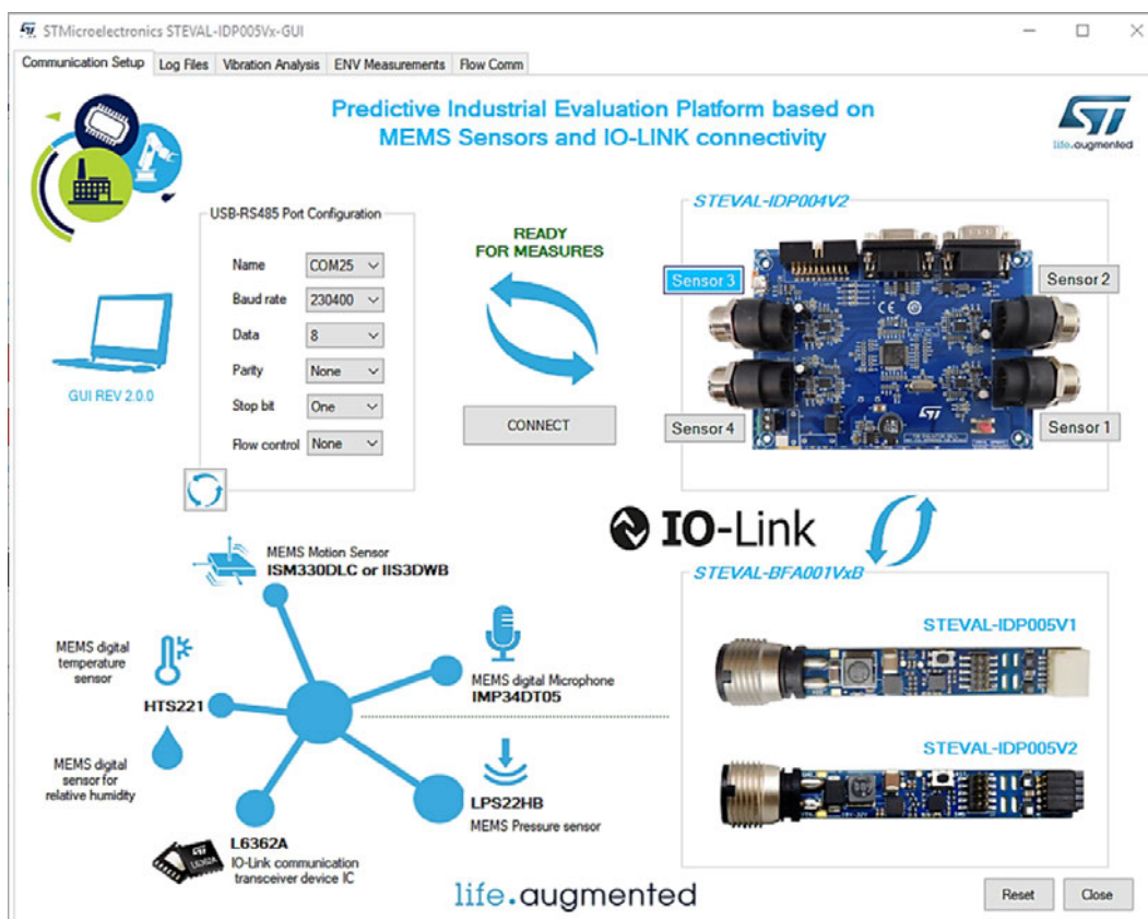
Figure 51. STEVAL-IDP004V2 and STEVAL-IDP005V2 connected and application start
