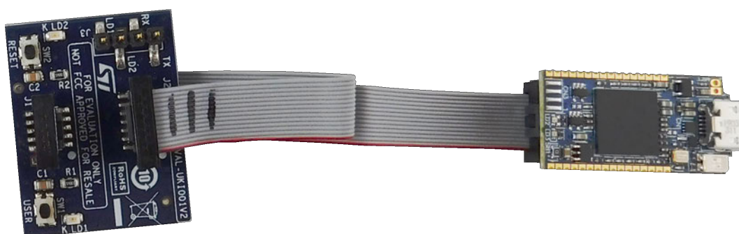
Figure 21. connection between STLINK-V3MINI and STEVAL-UKI001V2
