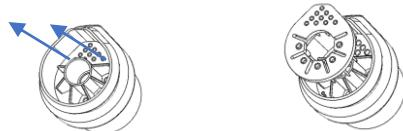
4. Solder wires to corresponding pin in insulator
