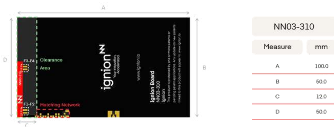
Figure 2 – PCB layout from Oxion TM
