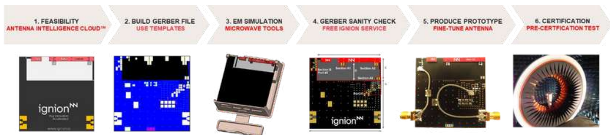
Figure 1 – Virtual Antenna® design journey steps for a successful IoT solution.
